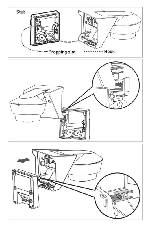
Mount the base plate on the wall / ceiling in the desired position by means of the supplied screw anchors.
