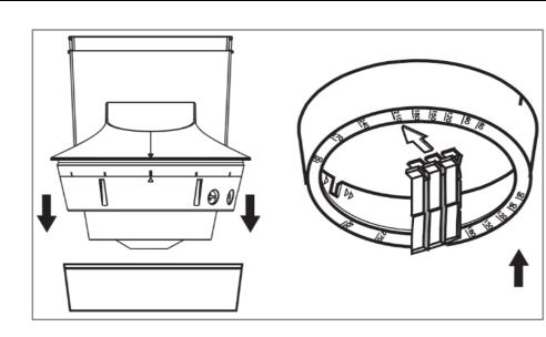
When the device is installed in place, make sure that the shield is in the correct position according to the required area masking.
