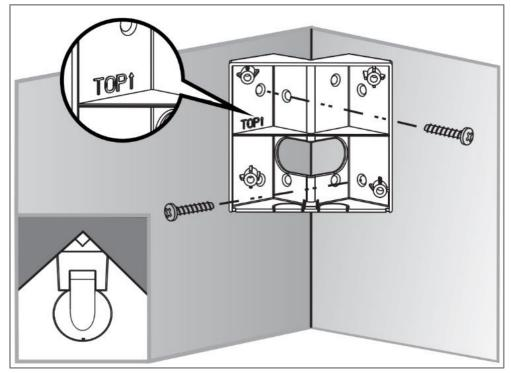
Fix the sensor body to the base plate securely through its own mounting screws and finally adjust the position of the sensor head.
