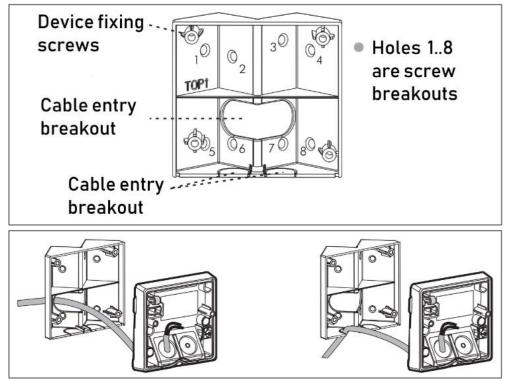
Fix the corner support on two sides either on an outer or inner corner.
