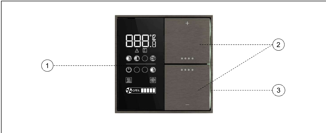
User interface: LC-display (1), rockers (2), LEDs (3) with lightguide
